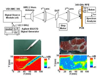
Fig. 4. Proposed THz transmissive imaging system.
