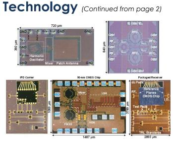
Fig. 3. Proposed THz receiver, V-band frequency doubler, and W-band packaged receiver.
